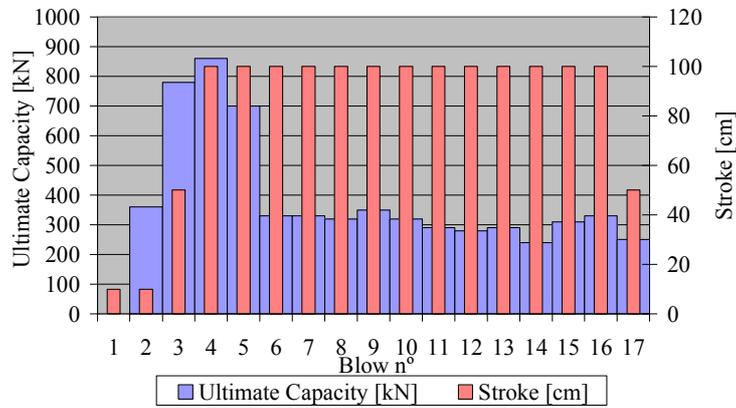
Figure 2. Ultimate Capacity: Micropile (5 m length) from CAPWAP and stroke per blow.
