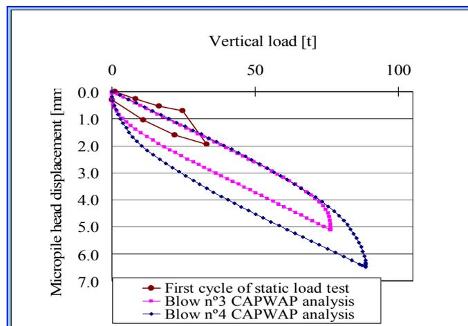
Figure 6. First cycle of static load test and CAPWAP static simulation for blows n°3-4.
