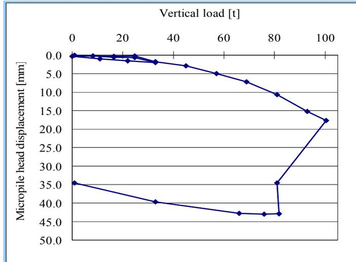
Figure 5. Static load test results on micropile.
