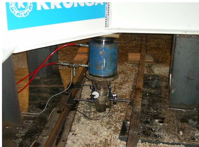
Photo 2. Hydraulic jack and reaction frame
