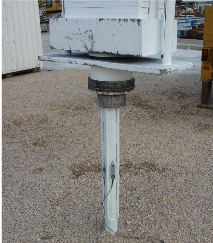
Photo 1. Hammer system and micropile with instrumentation.
