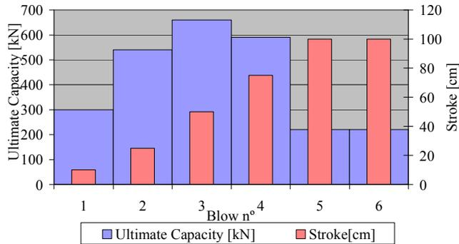
Figure 1. Ultimate Capacity micropile 3 m length from CAPWAP and stroke per blow.
