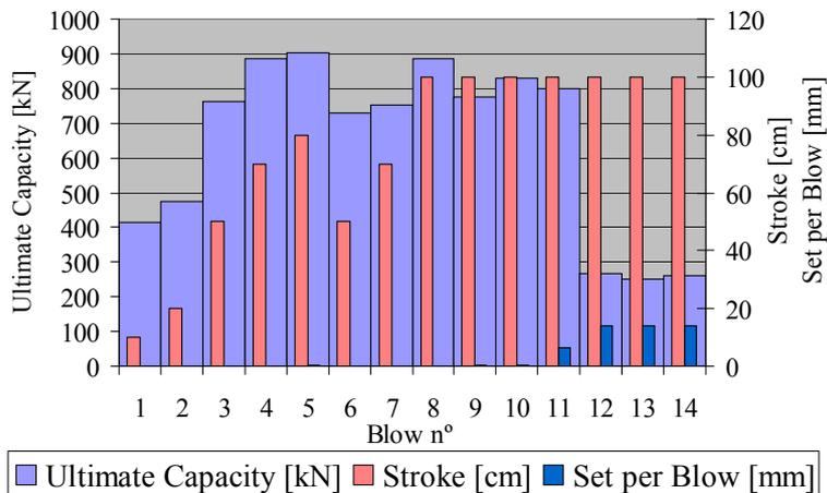
Figure 3. Ultimate Capacity: Micropile (7 m length) from CAPWAP and stroke per blow.
