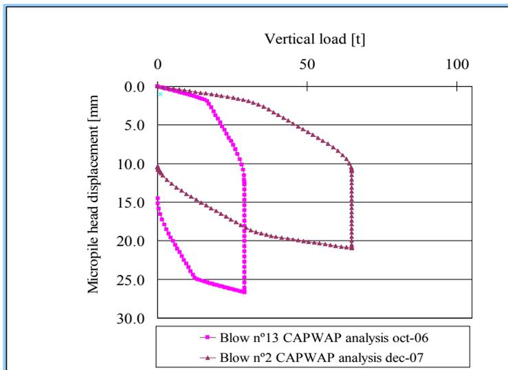
Figure 7. CAPWAP static simulation for blow n°13 (oct-06) and blow n°2 (dec-07)
