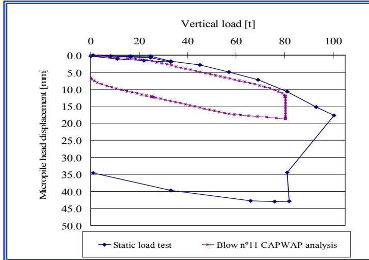
Figure 7. Static load test results and CAPWAP static simulation for blow n°11.
